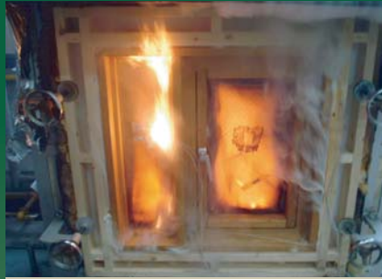
Fire protecting test on wooden sash
