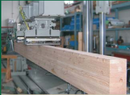
Flexural strength tests of actual-size material
