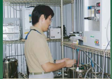
VOC measurement that uses small chamber
