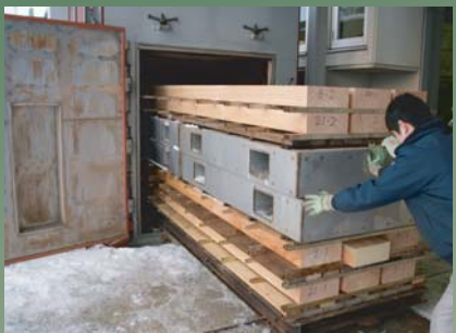
Experiments in artificial drying of wood
